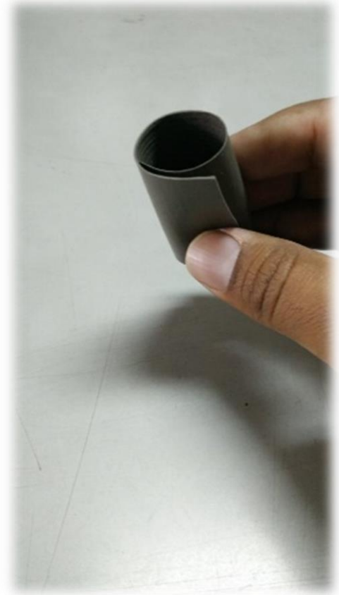
Figure 2 Flexibility of MoistureZero Cement Film
